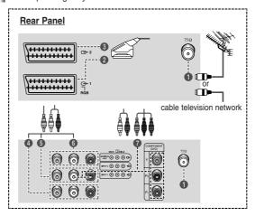
Whenever you connect an audio or video system to your television, ensure that all elements are switched off. Please be sure to match the color coded input terminals and cable jacks.
